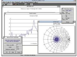
Use the Smith Chart for impedance matching of antennas and transmission line quality checks.
