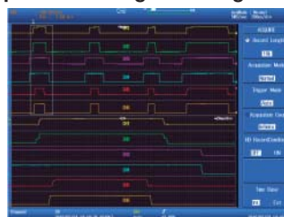
Example: Measuring inverter gate signals
