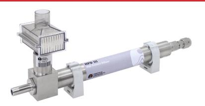
High Pressure Diffusers (HPDs) have been developed to address the challenge of sampling pressures of 5 – 100 psi, and the possible damage that can result from connecting pressurized air or gas to a particle counter. HPDs reduce the pressure of the gas to near atmospheric pressure by allowing some of the gas to diffuse out of the system, allowing the particle counter's flow-metering system to function as designed.
