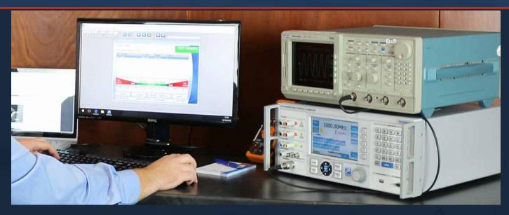
To expand the workload coverage of the 4000 Series calibrators a range of internal oscilloscope options are available.
