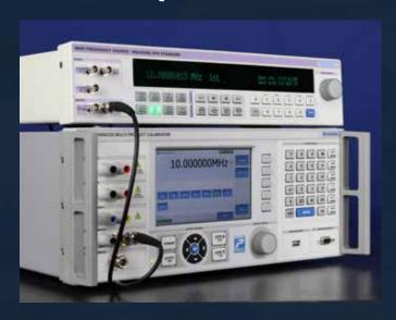
For calibration of high accuracy frequency counters, a 1ppm high stability frequency output is available (Included in 4010)
