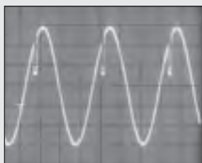
Sine wave with a dropout from 45° - 60°
