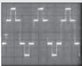
Six step sine wave
