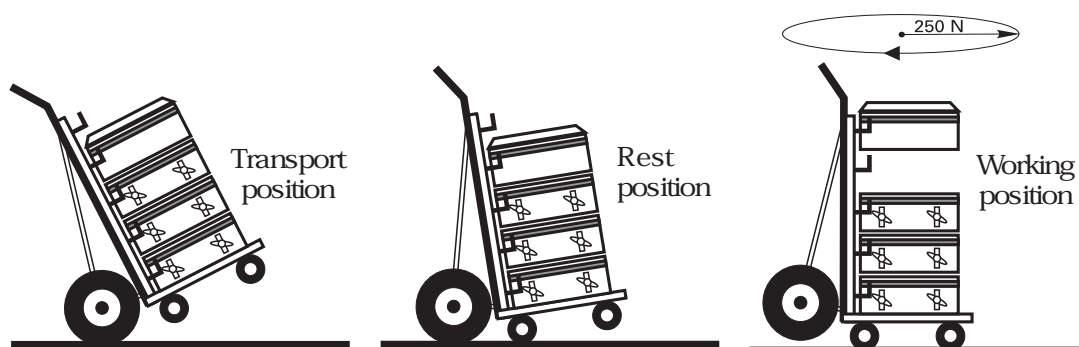
Fig 6.1 Different positions for the Oden AT carriage. Note, in working position the carriage must be secured to prevent tip over. Secure it to a suitable object e.g. a pole or a table.
