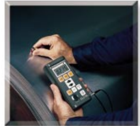
On-truck inspection of steel coils for confirmation to incoming QC specifications
