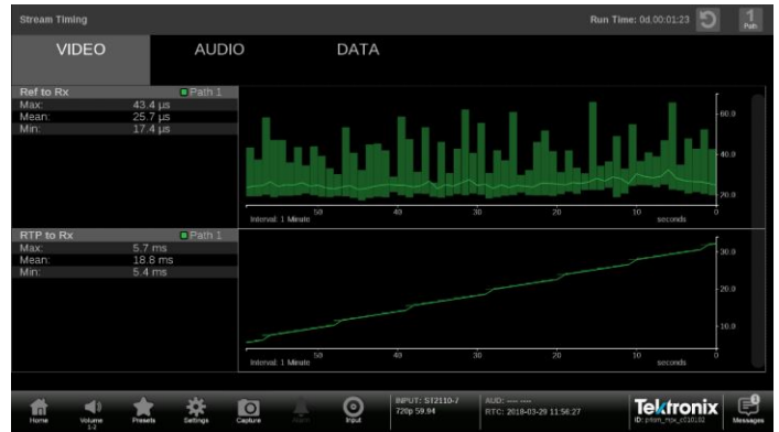
ST2110-20 timing against PTP and packet latency trend graph.
