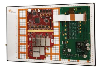
EMC and signal integrity are major concerns in the design of ultra-high speed (>2 GHz) PCBs. EMScanner enables the design engineers to diagnose EMC/EMI problems between 150kHz and 8GHz.
