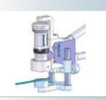
Support Z2 for thin cylindical parts, wires, bolts min. Ø 3 mm
