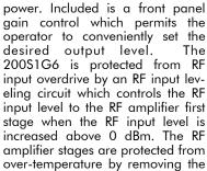
DC voltage to them if an over-temperature condition occurs due to cooling blockage or fan failure.
