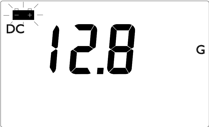
Figure 3-6 Low Battery Indication
