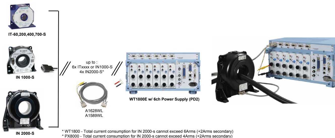
Figure 12 - Power analyzer with built-in power supply
