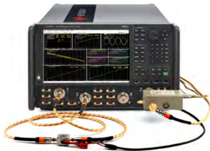
Keysight's NVNA software applications and accessories convert a Keysight 4-port PNA-X network analyzer into a high-performance nonlinear vector network analyzer.
