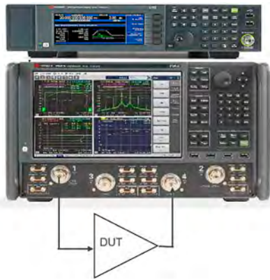
Classic NPR measurement with PNA-X and UXX
