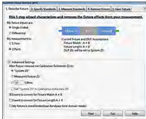
A five-step wizard guides you through the process to characterize your fixture and remove it from your measurement.
