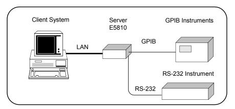
Thus, applications running on the computer system can transparently interface to GPIB and RS-232 based instruments over the LAN. Since several computer systems can access the E5810, groups of users can share access to the same GPIB and/or RS-232 instruments via the E5810. In addition, existing I/O applications that are supported with the E5810 and are designed for GPIB or RS-232 can use the E5810 without modification other than an address change.
