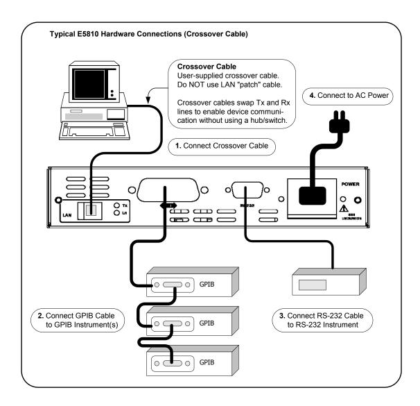
Apply Power to the E5810 After connecting the E5810 to a Local network, plug the E5810 AC power cord into an AC outlet and observe the power-on sequence. When the power-on sequence is complete, the default IP address of the E5810 is displayed on the second line of the front panel display. A typical display follows. See *Chapter 1*, "E5810A Description" for power-on sequences.
