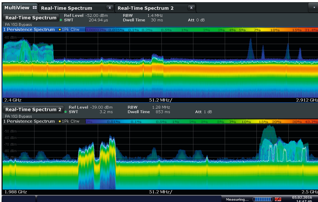
The persistence spectra 512 MHz above the ISM band at 2.4 GHz and below can be simultaneously displayed thanks to the MultiView function of the R&S®FSW.
