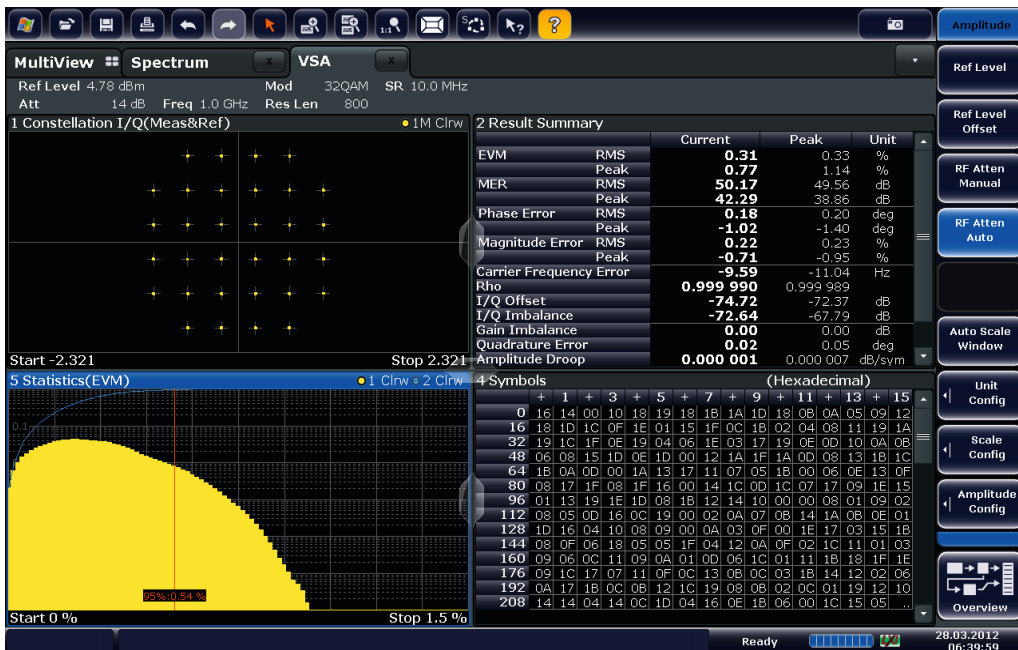
32QAM with four screens.
