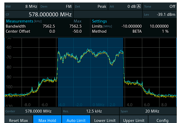
Automatic occupied bandwidth measurement of a DVB-T signal ( \beta % method).
