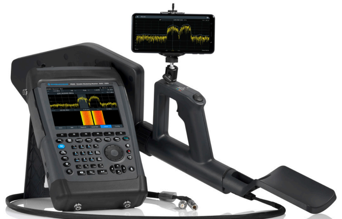
Interference hunting using the R&S®PR200 mobile app with gesture operation.
