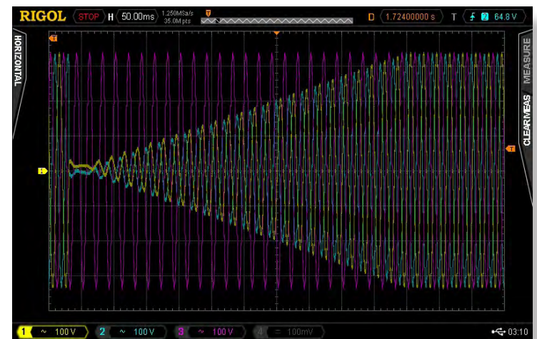
Figure 17: IEC 61000-4-34 Three Phase Voltage Variation Test
