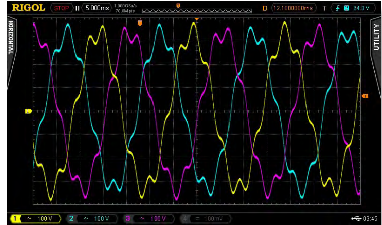
Figure 7: IEC 61000-4-13 Inter Harmonic Frequency Sweep Test
