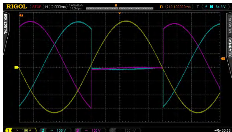
Figure 4: IEC 61000-4-11 1/2 Cycle Phase-to-Phase Voltage Dip
