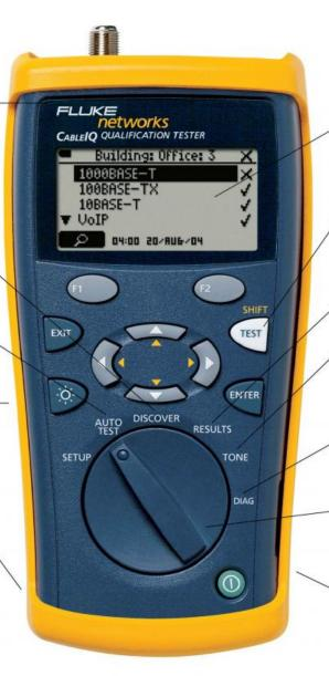
Graphical display. Backlit for viewing in all environments.
