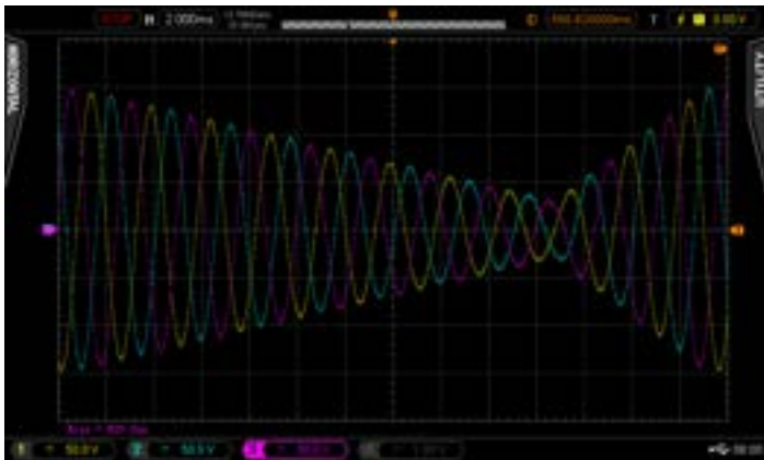
Figure 1: ABD0100.1.8 A380 Table A, Test Number 6, Three Phase Voltage Transient – short duration
