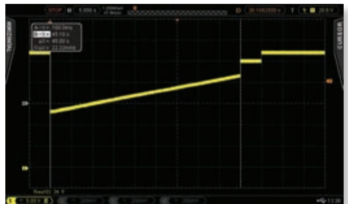
Figure 4: ABD0100.1.8E Table D, Test 7, A380 Heavy Load square DC pulse
