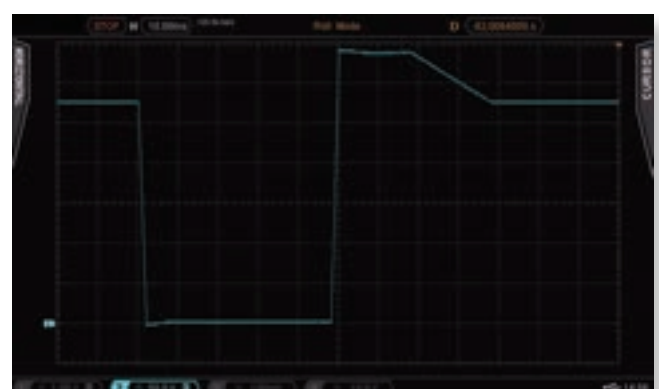
Figure 12: MIL-STD-704 Rev F, HDC 201 Cond K @ 10 mS/div – Detail
