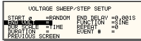
Figure 4-13: VOLTAGE SWEEP/STEP SETUP screen
