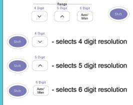
For increased measurement speed, select 4 digits. For increased accuracy, select 6 digits.
