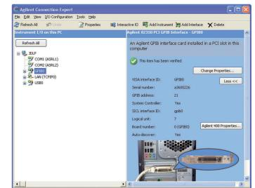
(4) Select the GPIB0 interface and then select the 34401A GPIB address (factory setting = 22).
