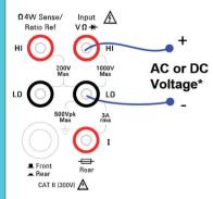
\* Also used for capacitance, continuity, diode test, frequency, 2-wire resistance, and 2-wire temperature measurements.
