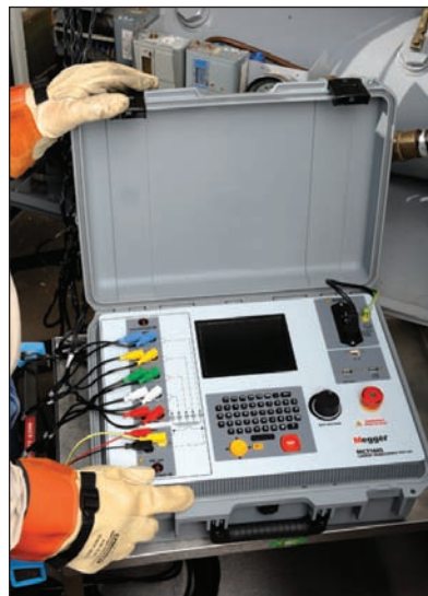
With a manual voltage output control knob, the user is able to perform any test required manually if only a spot check is required.
