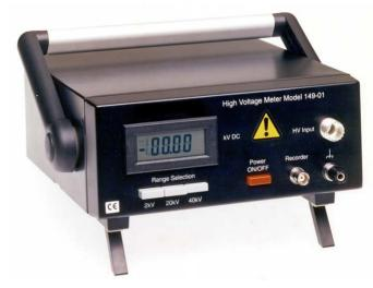
Caution: Great care must be taken when making measurements in high voltage circuits. Always ensure the HV return terminal of the meter is grounded. DO NOT use the hand-held probe on supplies that are potentially lethal.
