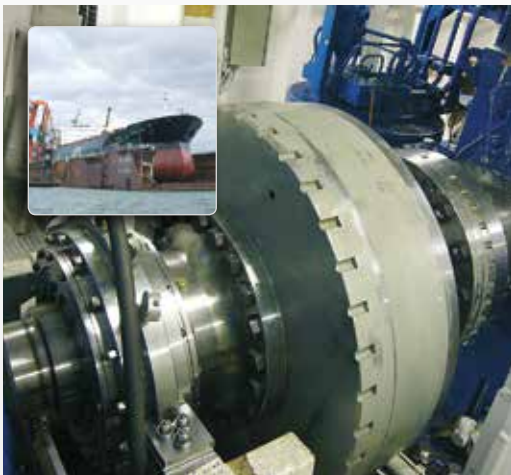
Engines, gearboxes and propeller shafts on ships are aligned using Easy-Laser® system. Thanks to versatile brackets you can install the equipment in the most appropriate place; shaft, coupling or flywheel.
