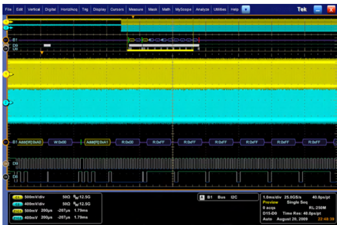
10 ms Duration Capture of Synchronous High-speed and Low-speed Signals at 25 GS/s.
