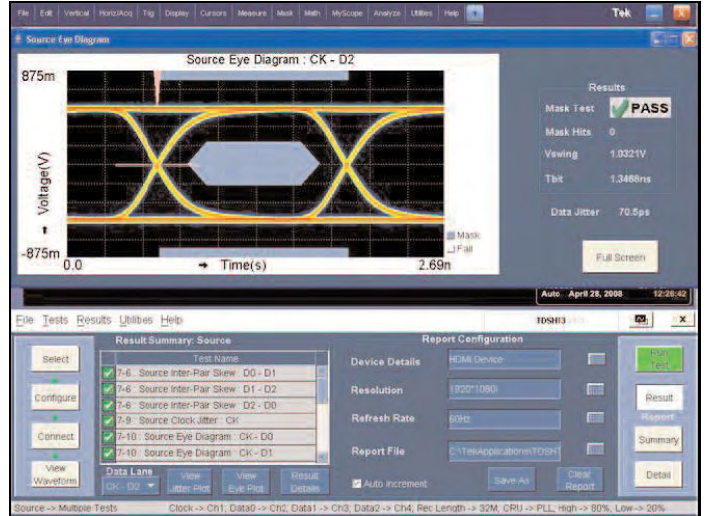
HDMI Compliance Test Solution (Option HT3) – Fast, efficient solution for HDMI compliance measurement challenges, no matter if you are working on a Source, Cable, or Sink solution. This application provides all the HDMI compliance test solutions you need to ensure quality and interoperability.
