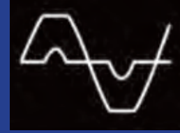
Oscillograph of voltage and current waveform at load due to distribution losses. THD=6.6%
