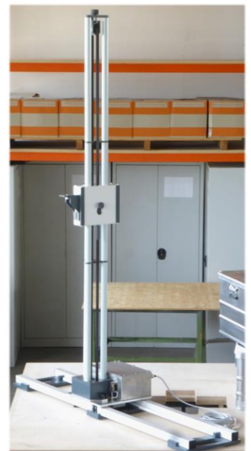
fig. 1: Field Probe Positioner FSM2315 in the 2014 version
