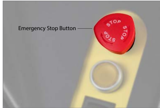
The Emergency Stop button.
