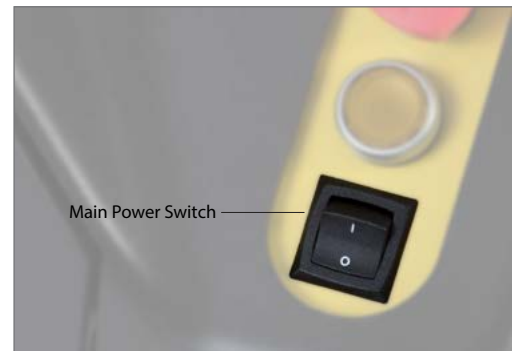
The Main Power switch.
