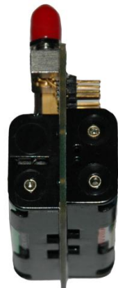
Vertical board with four batteries
