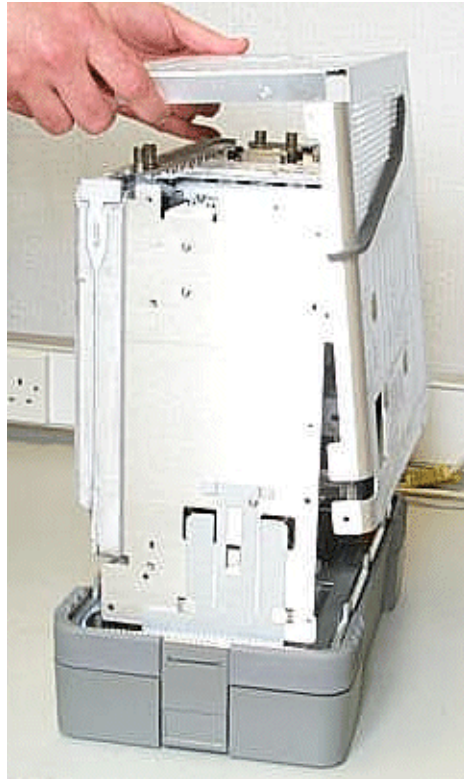
Figure 6-7 Chassis Cover Replacement
