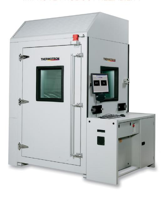
Thermotron's innovative Accelerated Stress Testing systems for Highly Accelerated Life Testing (HALT) and Highly Accelerated Stress Screening (HASS) find product failures fast with patented industry-leading technology. Performing HALT and HASS improves product reliability by maximizing lab efficiencies, all while reducing costs associated with warranties and recalls.
