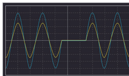
Voltage Interruption Loading Function
