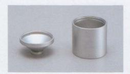
Glass Light-Projection Tube CR-A33f (For CR-300) and CR-A33e (For CR-310) Glass Light-Projection Tube CR-A33f and CR-A33e have a glass plate at the tip and can be used for measuring wet surfaces or for ensuring that materials such as textiles are flat during measurements.
