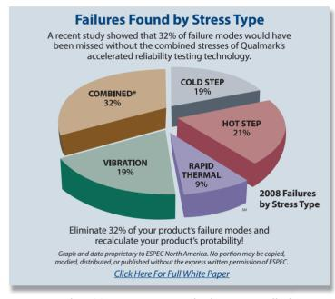
In HALT and HASS, stresses are applied in a controlled, incremental fashion while the unit under test is continuously monitored for failures. Once the weaknesses of the product are uncovered and corrective actions taken, the limits of the product are clearly understood and the operating margins have been extended as far as possible. The result? A more mature product can be introduced much more quickly with a higher degree of reliability.
