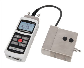
FS05 force sensor connected to an M51 indicator via AC1083 adapter for off-site calibration
