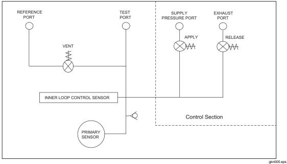
Figure 2-4. RUSKA 7250 Absolute Pneumatics Diagram 3000 PSIA (20.7 MPa) FS
