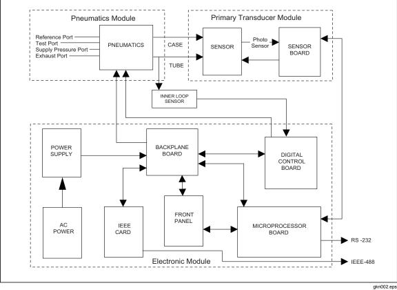
Figure 2-1. Calibrator Block Diagram
