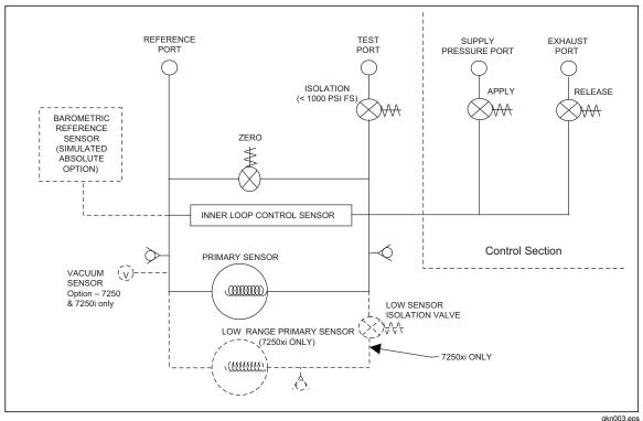
Figure 2-2. RUSKA 7250 Gauge Pneumatics Diagram 5 to 2500 psig (34 kPa - 17.2 MPa) Full Scale Ranges
