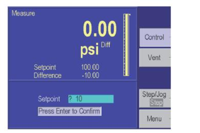
will appear below the scratch pad. Notice that the upper left corner still shows MEASURE. The Calibrator stays in Measure mode until the change is confirmed.
