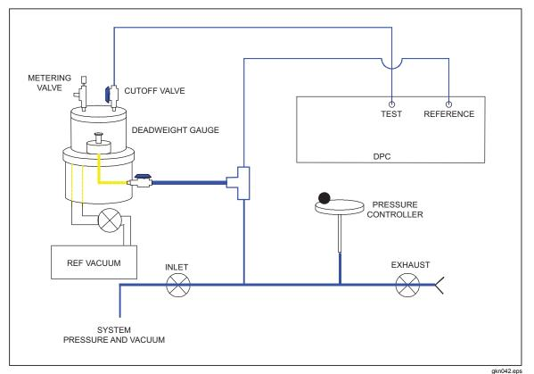
Figure 6-3. Vacuum Calibration
