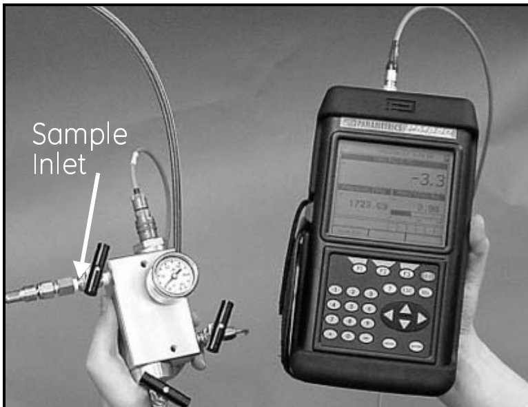
Figure 2-1: The Sample System and the PM880
