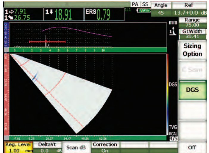
Phased Array DGS/AVG Mode
