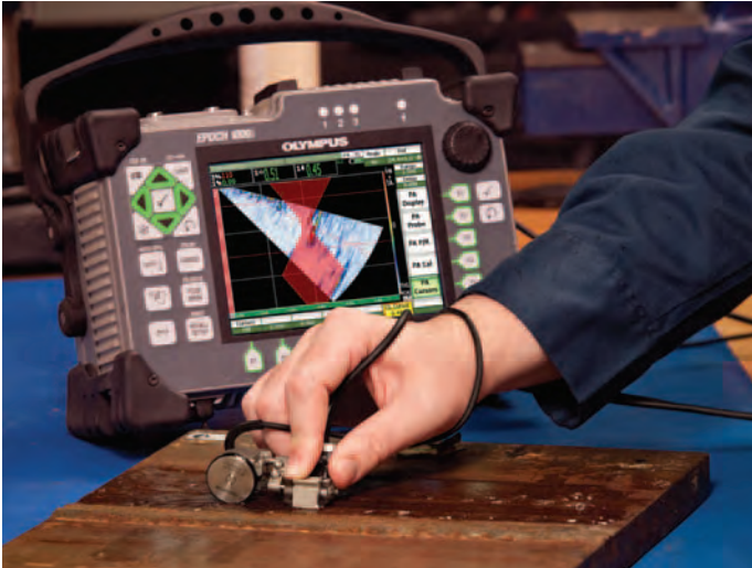
Phased Array S-scan with Weld Overlay
