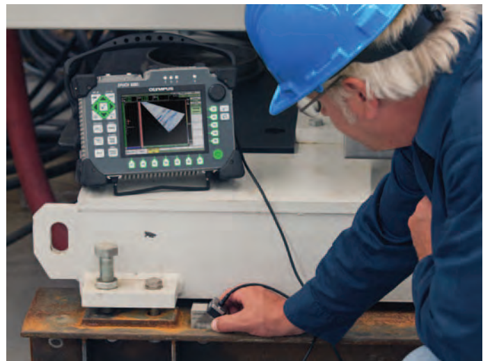
AWS “D” Weld Rating displayed for 45° focal law
