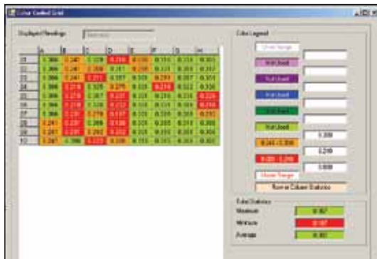
When viewed on your PC a color coded grid easily flags out-of-tolerance thickness conditions.
