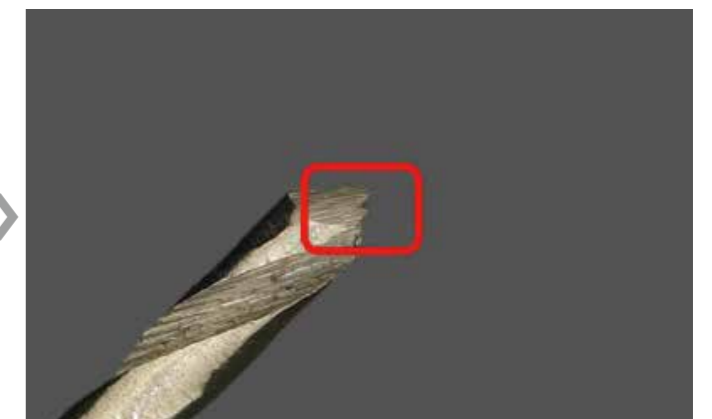
Easy observation (24X) of damaged area with DSX1000 thanks to the flat lighting
