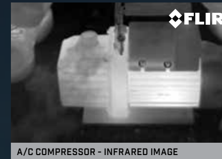
A/C COMPRESSOR - INFRARED IMAGE
