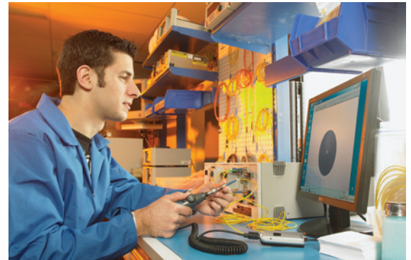
Patchcord inspection in a manufacturing environment
