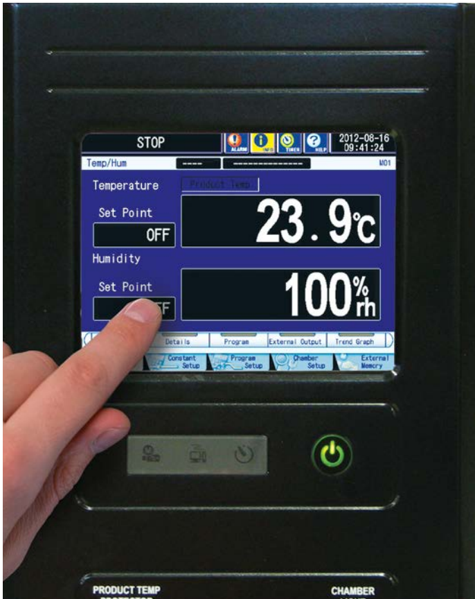
The console includes the P-300 programmer, USB port, product temperature protector, and chamber light (option).
