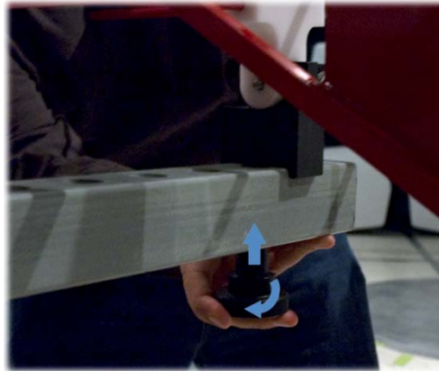
Non-stinger method to mount Model 3143B to 7-TR
